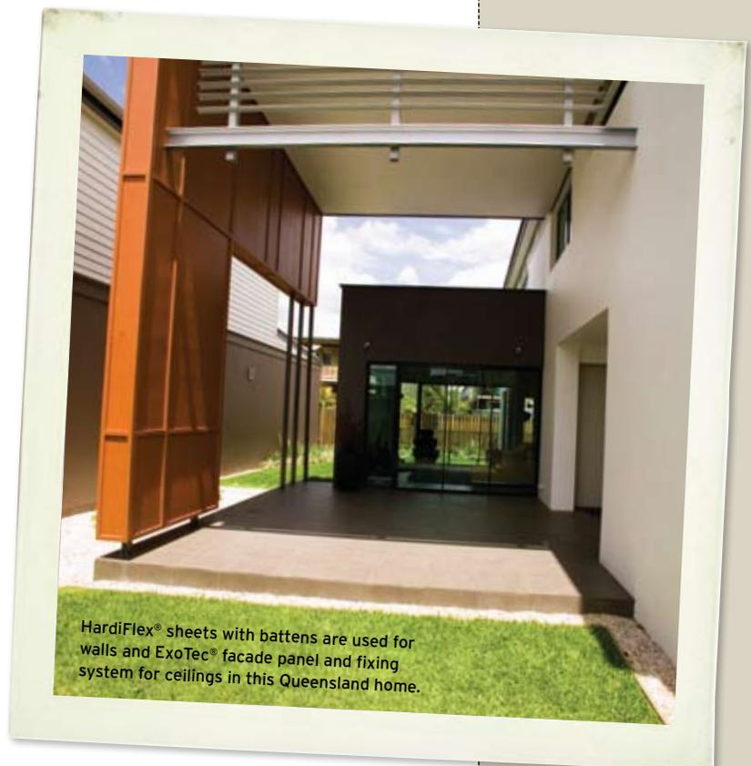
HardiFlex® sheets with battens are used for walls and ExoTec® facade panel and fixing system for ceilings in this Queensland home.
